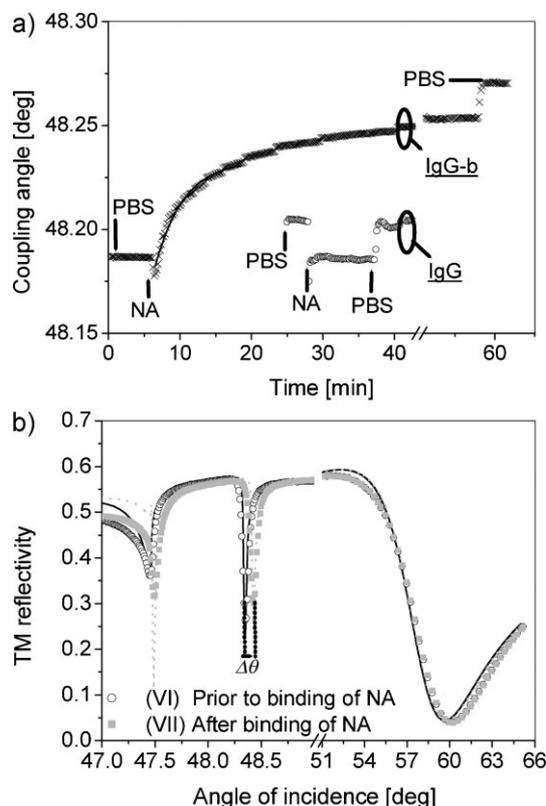
Figure 3. A) Time evolution of the  $\text{TM}_1$  coupling angle showing the binding of NA to a gel modified with IgG-b and IgG. B) Measured reflectivity spectra before (circles) and after (squares) the affinity binding of NA with corresponding fits (lines).
