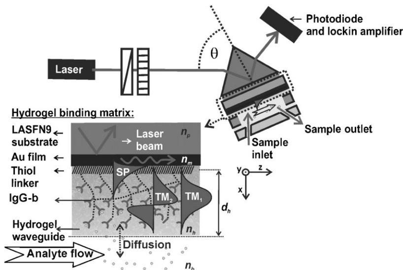
**Figure 1.** Optical setup for the excitation and interrogation of guided waves within a thin hydrogel film.
